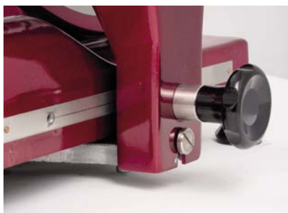
Carriage with locking mechanism
