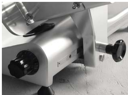
Carriage with locking mechanism
